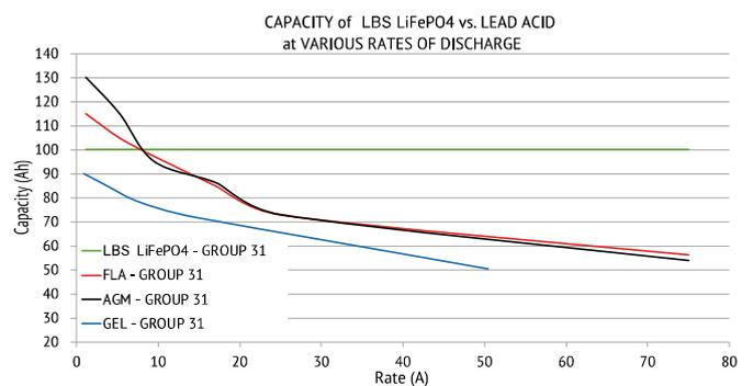
\* The curve is only the reference of the comparison of discharge performance of Group31 batteries with different materials, might not for the specific model in the specs.
